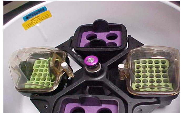
Sealed rotor heads or centrifuge safety cups
